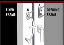
Position the lock unit (A) on the opening frame and the cable unit (B) on the fixed frame. Directly screw provided self-drilling screws with a crosshead screwdriver.
