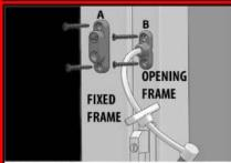
Position the lock unit (A) on the fixed frame and the cable unit (B) on the opening frame. Directly screw provided self-drilling screws with a crosshead screwdriver.
