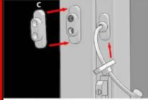
Clip plastic covers (C) in to position over the lock and the cable unit. Once clipped, they can not be removed easly, please do not try it before installation.
