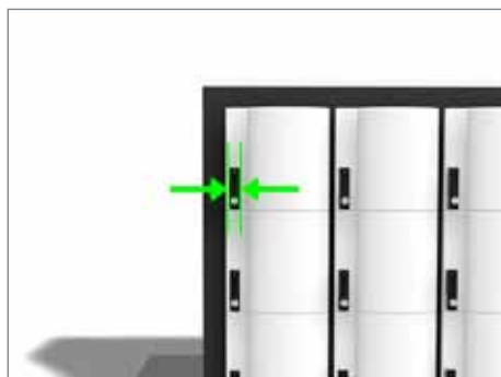
Example: Cabinet doors that curve outwards
